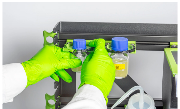
A laboratory threaded bottle is removed from a holder module with retaining ring from a SmartRack® classic.
